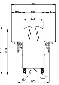
D Drain = = Electrical inlet (power) EI
